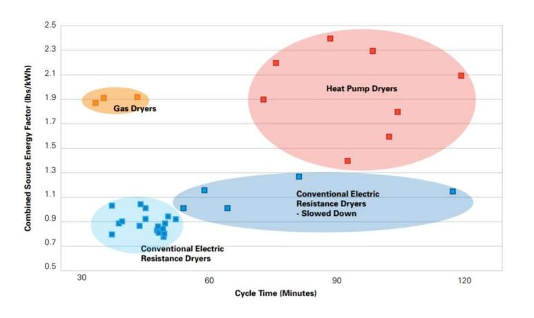
Heat pump units average 36% savings over standard clothes dryers vs. 22% savings for efficient clothes dryers
